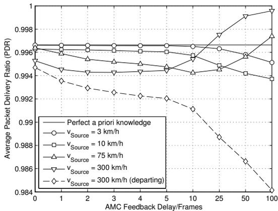
Fig. 7. Average packet delivery ratio (PDR) versus AMC feedback delay.
