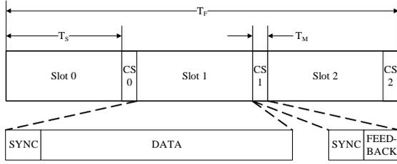
Fig. 2. TDMA frame structure consisting of data slots and control minislots (CS) for AMC feedback information and other control data.
