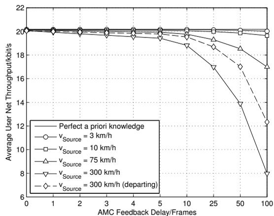
Fig. 5. Average user net throughput versus AMC feedback delay.
