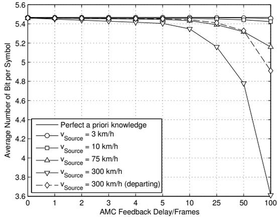
Fig. 6. Average number of bits per symbol (coding not considered) versus AMC feedback delay.
