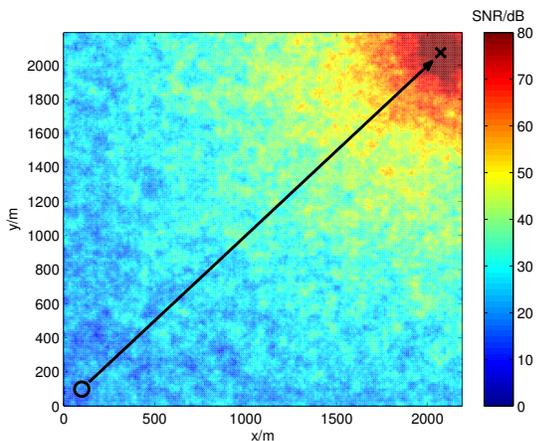
Fig. 4. Overview of simulation scenario;  $o$  and  $x$  represent the initial positions of the source and destination node, respectively.
