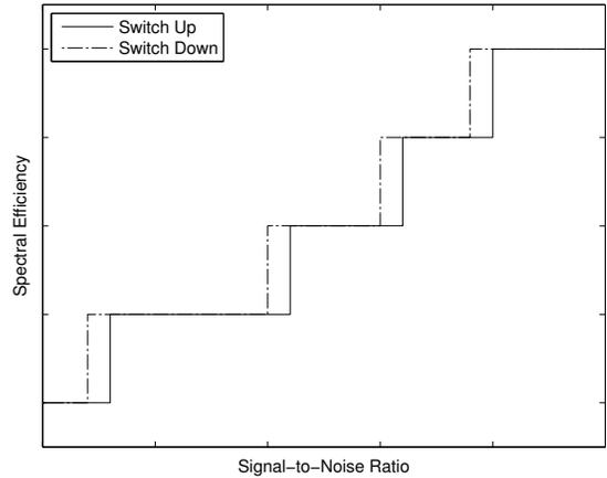
Fig. 3. Qualitative representation of thresholds for AMC.
