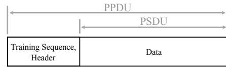
Fig. 4. Structure of a TDMA-slot.
