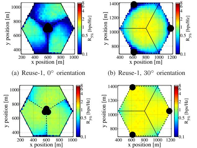
Fig. 3. Cooperation of 3 BSs: 5% outage rate, reuse-1 or FDMA.
