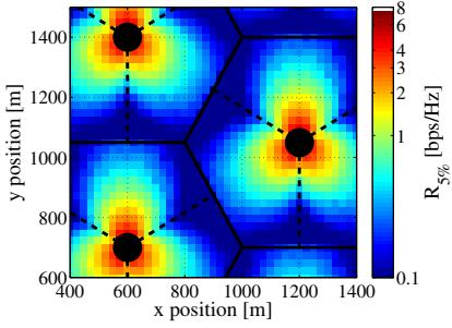
Fig. 2. Reference scenario 5% outage rate: no cooperation, no handoffs, FDMA, 0° cell orientation (a).
