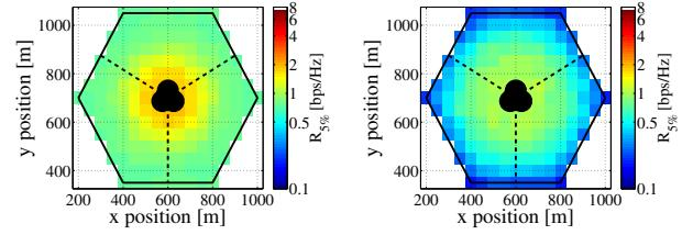
(a) MU-MIMO macro diversity (b) MU-MIMO joint beamforming
