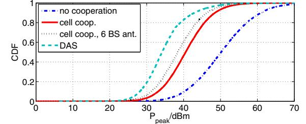
Fig. 7. CDF of max. Tx power of 3 cooperating BSs, target rate 1 bps/ Hz, reuse-1, 30° orientation (BSs with  $N_B = 6$  as reference for the DAS case).
