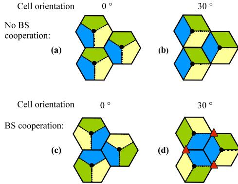
Fig. 1. Investigated cell orientations. For FDMA, the colors indicate sectors using the same frequency band. Red triangles in (d) mark the positions of supporting nodes in case of a distributed antenna system (DAS).
