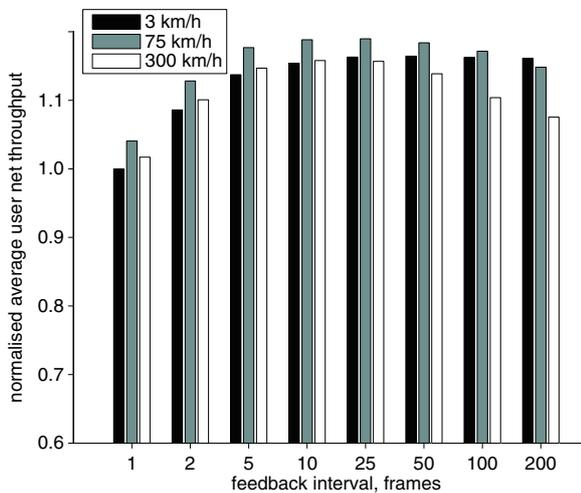
Fig. 2 Normalised average user net throughput against CQF interval for link adaptation starting in steady state
