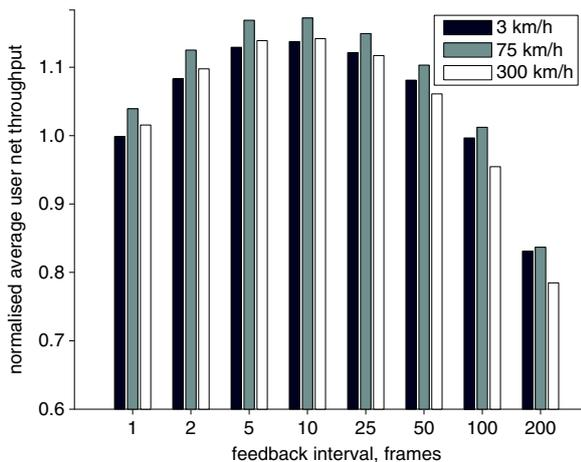
Fig. 3 Normalised average user net throughput against CQF interval for link adaptation starting with basic MCS
