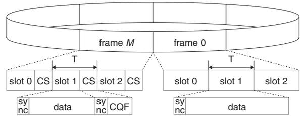
**Fig. 1** TDMA superframe structure consisting of  $M+1$  frames. Frames 0 to  $M-1$  accommodate data slots only, whereas frame  $M$  consists of both data slots and CS for CQF
