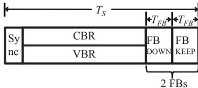
Fig. 4. TDMA slot structure of the proposed FR-2Slot mechanism.
