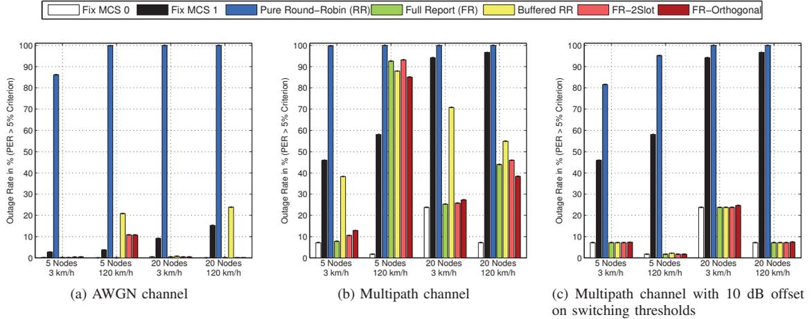
Fig. 7. Outage rate for PER > 5% in AWGN and multipath channels for different scenarios (velocities and number of destination nodes).
