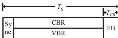
Fig. 5. TDMA slot structure of the proposed FR-Orthogonal mechanism.
