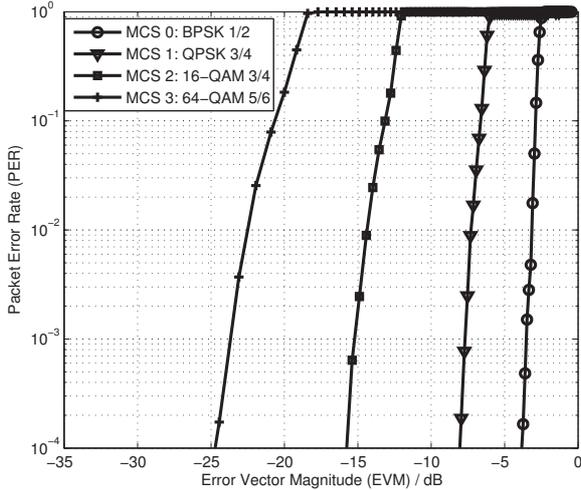
Fig. 2. PER of the considered narrowband system versus root mean square error vector magnitude (EVM).
