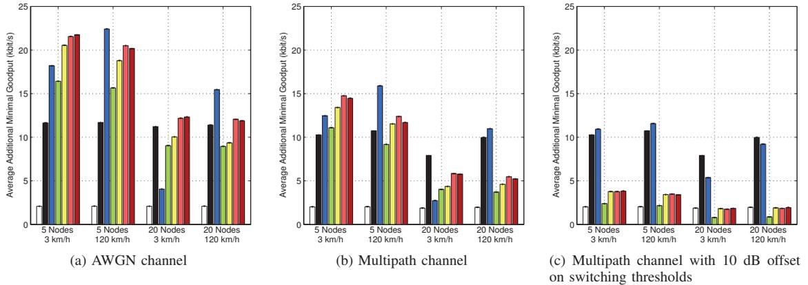
Fig. 8. Average additional minimal goodput in AWGN and multipath channels for different scenarios (velocities and number of destination nodes).
